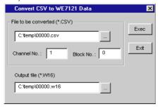
3. Enter the name for the converted file in the [Output file] entry box, and click [Exec]. The file extension of the converted file is ".w16."
